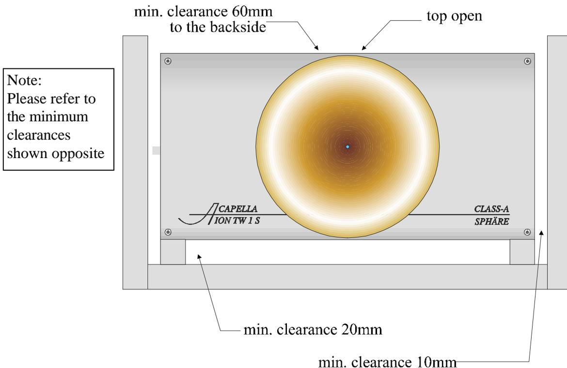
During installation in a cabinet, the above mentioned minimum clearances must be observed. Be sure to allow perfect heat dissipation through vertical air circulation. Besides, the rear side of the cabinet must have an air inlet corresponding to the width of the tweeter. No objects which could hinder free air circulation should be fitted above the tweeter. As a freestanding unit, a 10 mm minimum clearance between the bottom-panel of the unit and the base will be sufficient.
